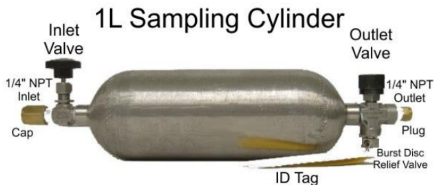
Figure 7-3: Example of double-ended sample cylinder (Atlantic Analytical Laboratory, 2021).
